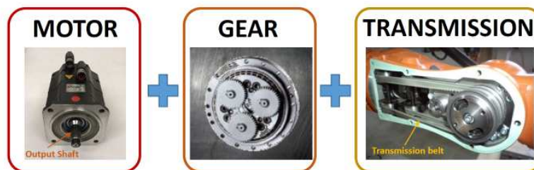
Figure 8.3-4 Examples of robot electrical motor, planetary gearhead and belt transmission*. Image rights: Dr. Arun Dayal Udai.
